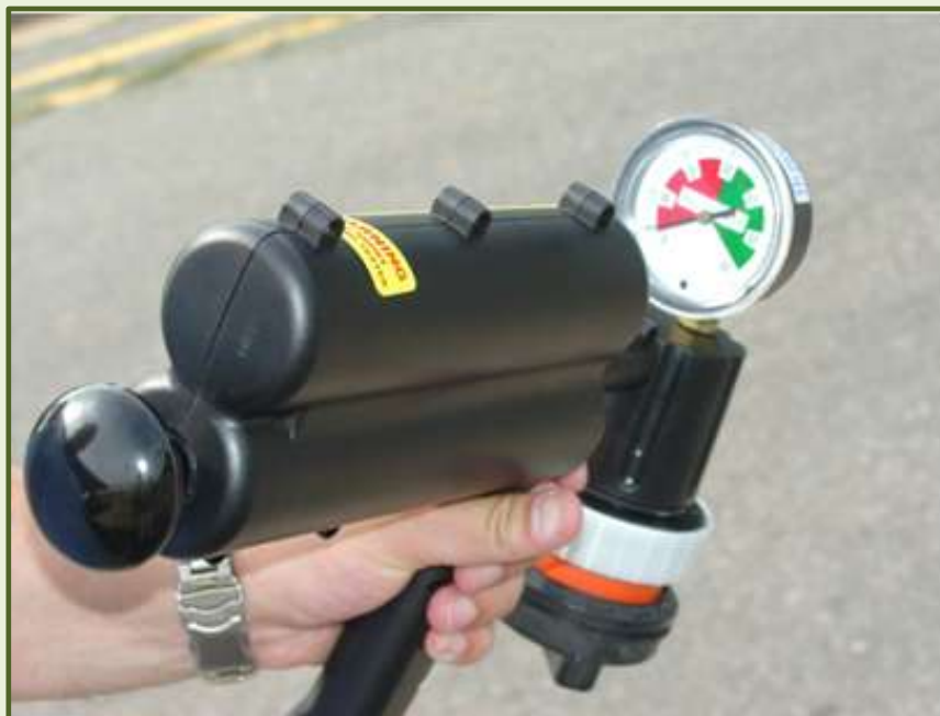
The vehicle's gas cap is attached to a device that determines the leakage rate of the cap in under a minute
