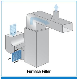
Furnace or HVAC filter—Select a filter rated at least MERV 13 or as high as your system will accommodate.
